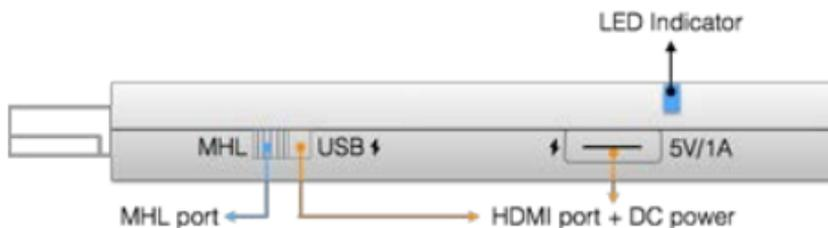
The EZCast Pro dongle is compatible with MHL interface, so there are 2 ways to connect with EZCast Pro dongle with your receiver devices like TV, Monitor or Projector. Use the switch to choose HDMI output or MHL output, please be noted your MHL device must provide 900mA power, and if you use HDMI out, you will need external 5V/1A DC power to bring up the dongle.
